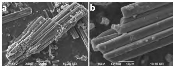
**FIGURE 1.** SEM image of bundle rapidcreekite crystals (a) and details showing the EDS-confirmed carbonate phase growing on their crystal surface (b).
