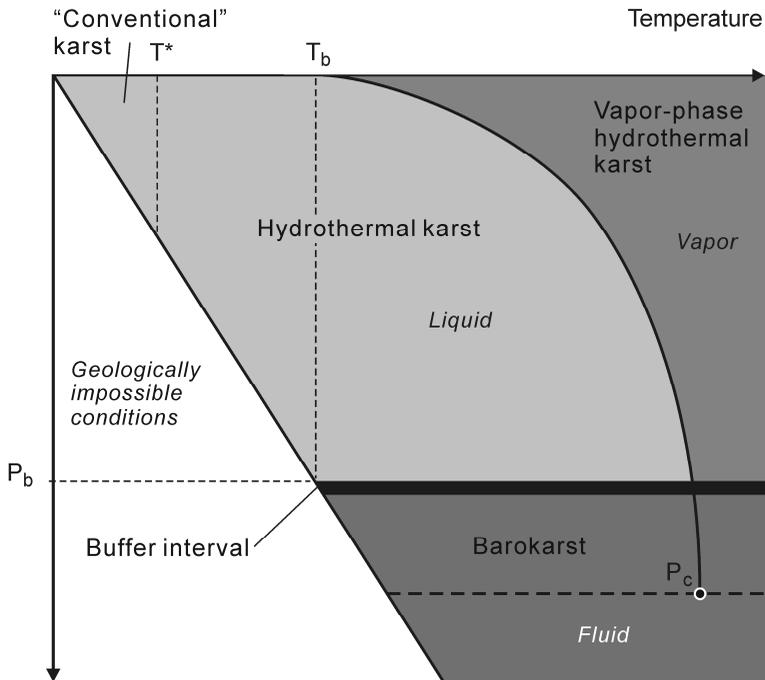
**Fig. 5.** Boundary condition of karst in the Earth's crust:  $P_c$  – critical point for water;  $T^*$  - conventional minimum temperature of thermal water;  $T_b$  – temperature at buffer interval (empirically determined; 80-100°C);  $P_b$  – pressure equal to the tensile strength of rocks.
