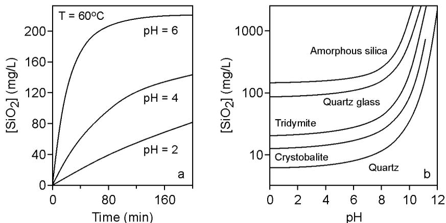
**Fig. 1.** Solubility of SiO<sub>2</sub> in water in different conditions (according to Mitsiuk, 1974): a – the dissolution rate of amorphous SiO<sub>2</sub> at T = 60°C and varying pH; b – solubility of different varieties of silica with change of pH in standard conditions.
