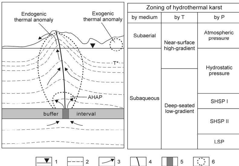
**Fig. 4.** Zoning of hydrothermal karst in the Earth's crust: 1 – water table; 2 - isotherms; 3 – flow direction; 4 – axis of enhanced-permeability zone; 5 – hydrofracturing of the buffer interval; 6 – areas of "anomalous" hydrothermal karst and area of the anomalously high aquifer pressure (AHAP). T\* - conventional minimum temperature of thermal water; SHSP I – suprahydrostatic pressure; SHSP II suprahydrostatic pressure exceeding the tensile strength of rock; LSP – lithostatic pressure.
