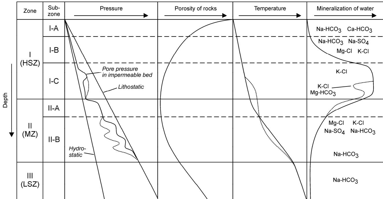
**Fig. 2.** Scheme of the vertical hydrodynamic zoning of the Earth's crust showing changes in some important parameters (after Ezhov & Lysenin, 1986; 1988): Solid line – parameters before the impulse breakthrough of fluids through buffer sub-zone II A; dotted line – parameters after the breakthrough. Definitions of zones and sub-zones are given in text.
